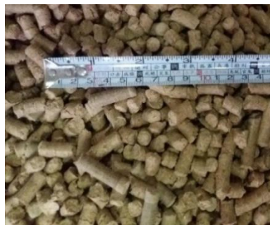
Briquetting and pelletizing from rice straw
