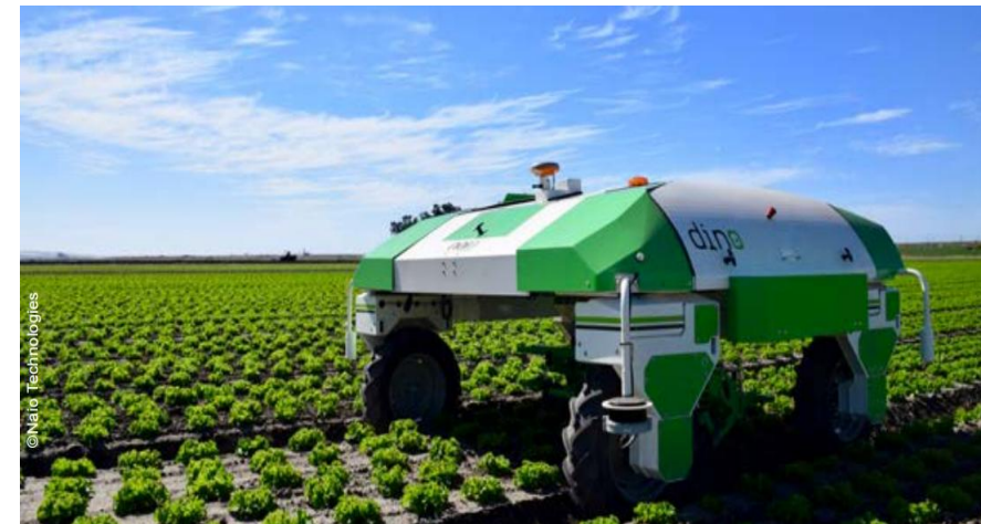
Self-powered platform (Agrointelli, Denmark)
