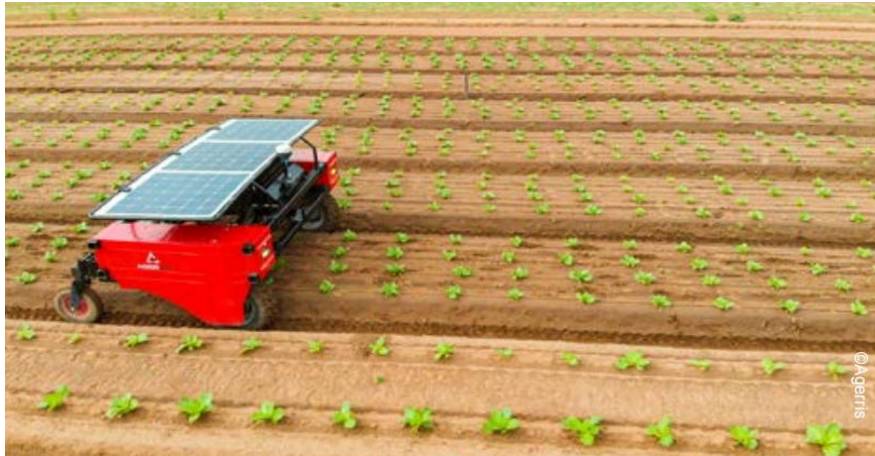
Solar-powered robot (Agerris Farmhand, Australia)
