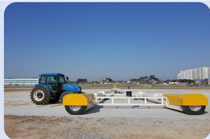
Harsh surface Durability test system
