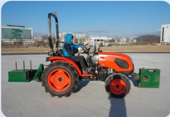
Steering emergency mode check ISO 789-11
