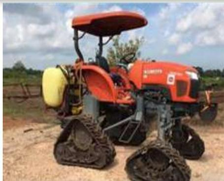
4 half track tractor- rubber typed
