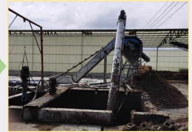
Separation of biogas residue and slurry
