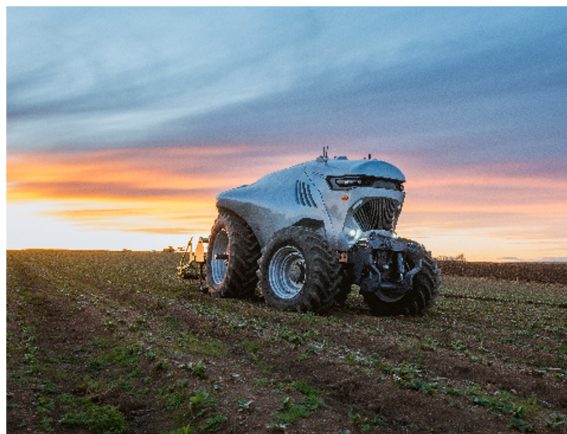
“Honghu” smart agricultural machinery released by the Chinese Academy of Sciences in Dahewan of Heilongjiang province, September 2022. The equipment comes with a smart electric control system and automatic driving system and can perform whole-process smart operations through the smart control system for field operations. The power of its main drive motor is up to 300KW.
