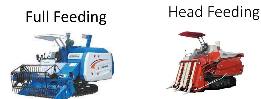
Combine Harvesters can be divided into full feed and head-feed depending on the feeding method. The difference between the two is that the full feeding is to send the cut straw and the head to the threshing drum for threshing. Head-feeding is to send only the head/ panicles to the threshing drum for threshing. The first consumes a large amount of power and broke straw. The second only threshes the head, which consumes less power, but the structure is more complicated, and keep whole straw.
