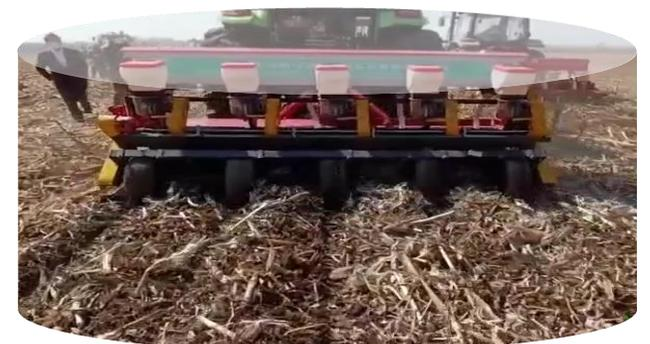
Use powered knife to do strip till and make a clean zone for the coming sowing
