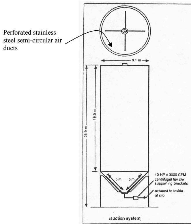
Figure 2. Aeration ducts configuration for the modified MFR ( $0.1 \text{ m}^3/\text{min}/\text{t}$ )
