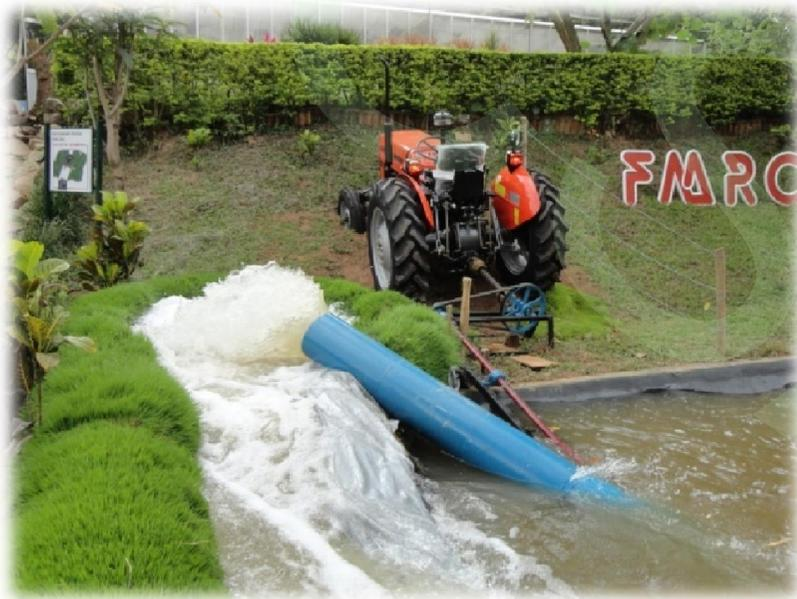
“ Very high capacity (more than 20,000 l/min.) four wheel tractor powered axial flow type water pump has been developed. It has very good demand in the Eastern Province. A number of manufacturers in that province were already trained. It consumed very low fuel per liter of water.
