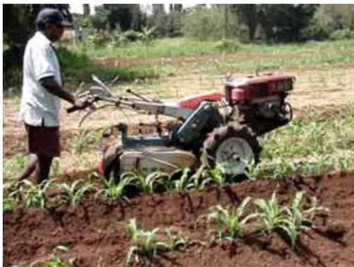
Use of two wheel tractor rotary as an inter-cultivator
