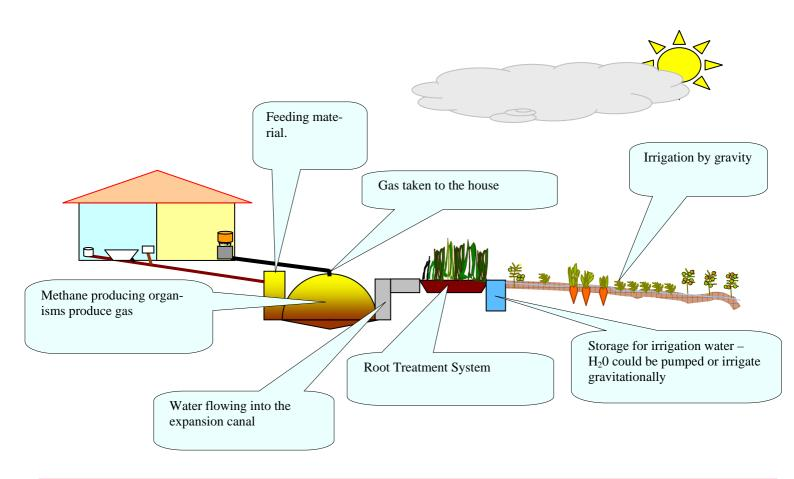
**Sketch of biodigester replacing a septic tank**. Wastewater as well as kitchen and garden waste enter the digester and are broken down to biogas and fertile water.
