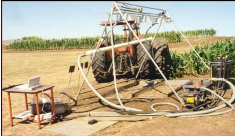
Fig.1 A portable rainfall simulator with two tipping buckets connected to a laptop computer.
