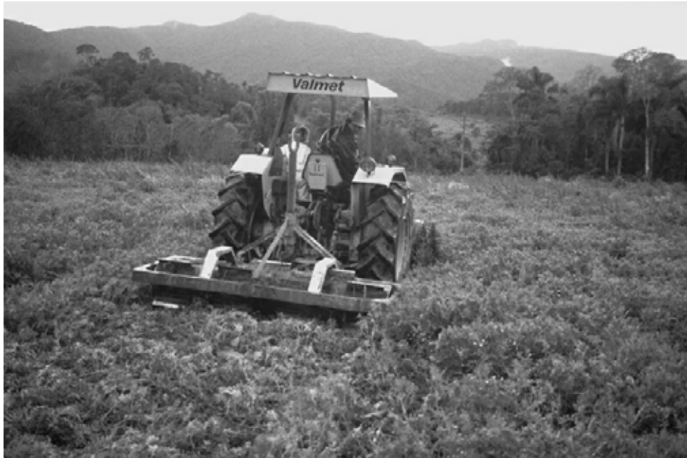
Picture 1: Knife roller used for rolling down a cover crop (photo by Friedrich).
