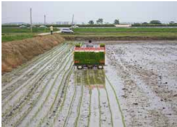
Map-based variable fertilizer applicator attachable to a transplanter
