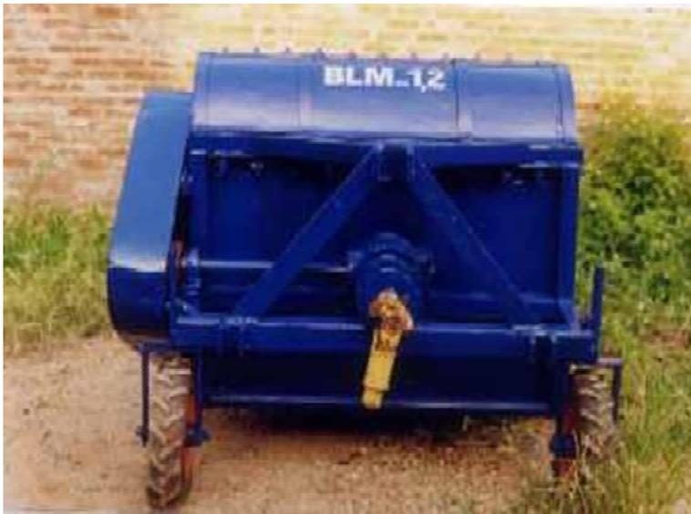
*Fig. 4. Sugar-cane-leaf rotary chopper
