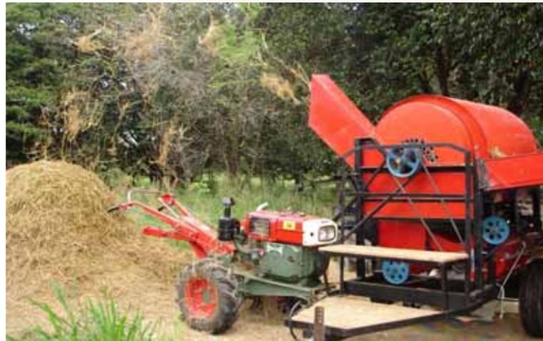
High Capacity Thresher for 12 hp Power Tiller
