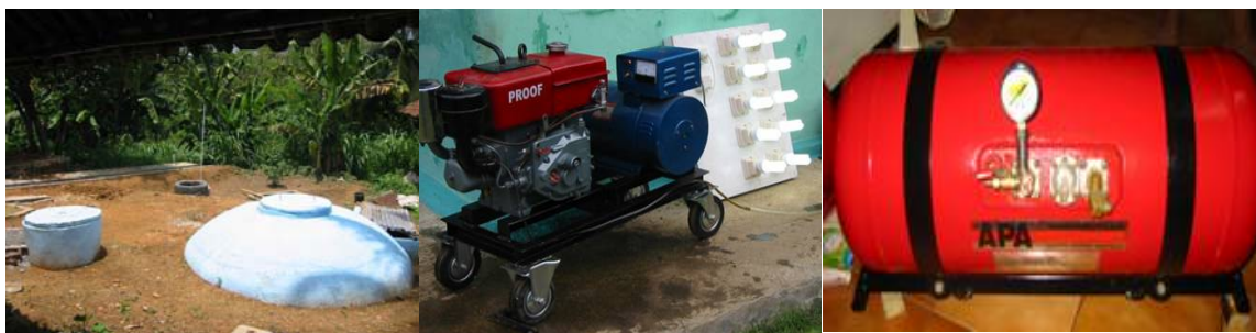
Figure 4. Biogas reactor, dual-fuel engine for electric generator and biogas bottling
