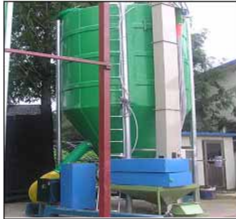
Fig. 4 Natural air drier-cum-low temperature storage bin
