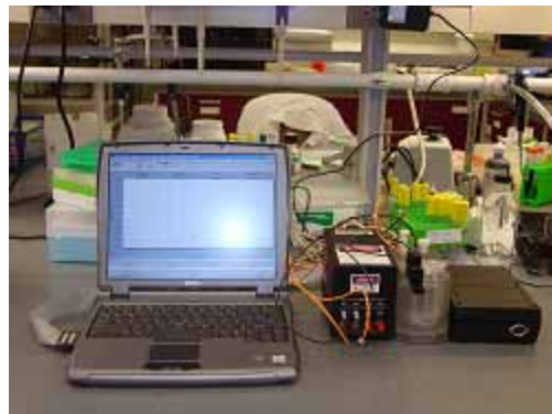
Fig. 25 Fiber-optic bio-sensor for Salmonella detection
