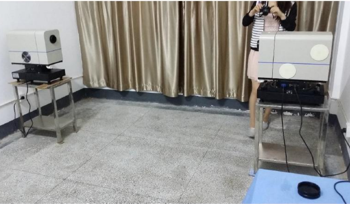
An alternative droplet sampling complete with a droplet analysing software based on light diffraction
