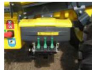
Induction hopper for loading chemical products
