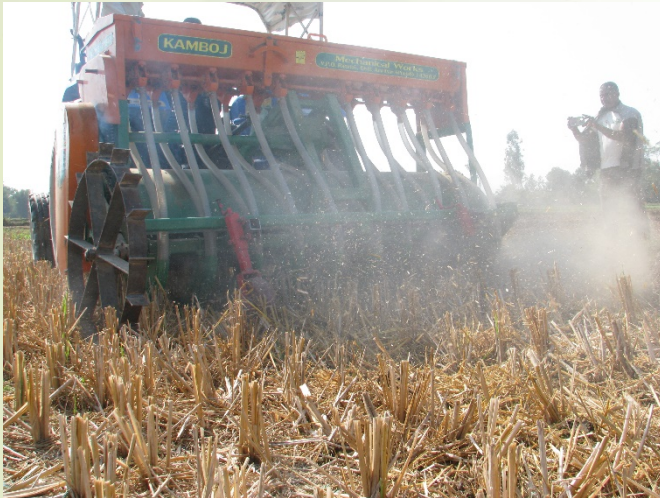
Fig 1: Use of Happy Seeder over left residue by Combiner
