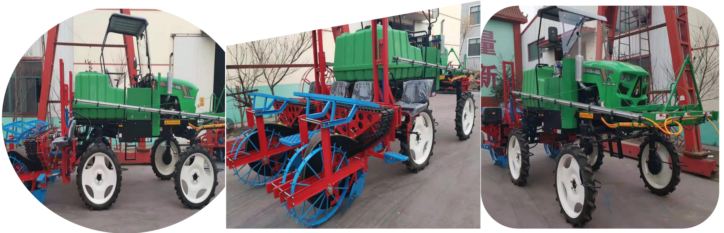
Multifunctional machine for plant protection, fertilization and transplanting
