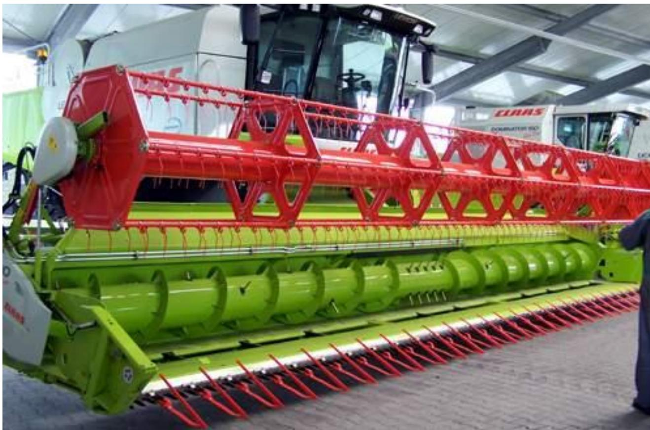
**CLAAS harvester with a cutting width of 9 meters**
