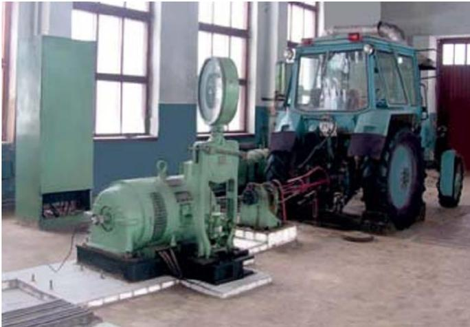
Test engine power up to 400 kW
