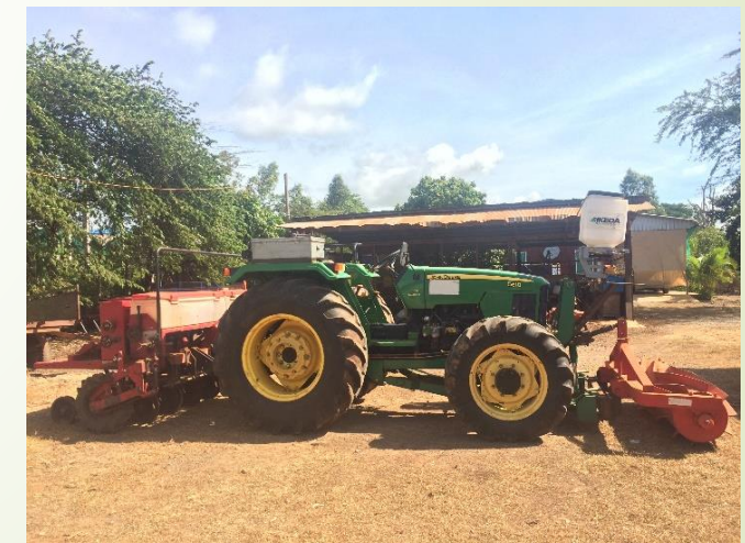
NT planter, broadcaster & roller crimper
