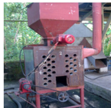
Figure 18: AMDP Rice Husks Furnace for Fruits and Grain Drying
