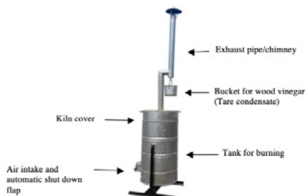
Figure 2: The Picture Shows the Top- Lit Up-Draft (TLUD) Kiln with Some Design Features.
