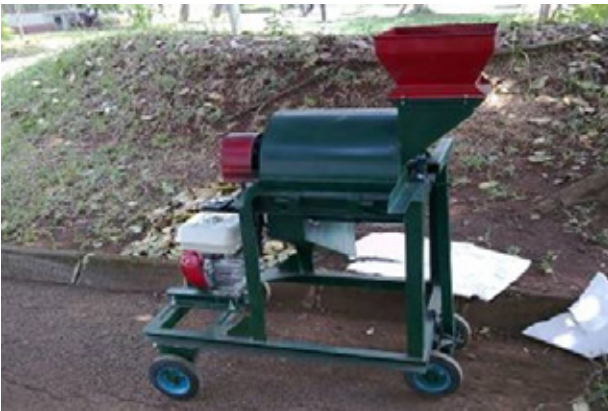
Figure 4: Hammer Mill of 500 kg/h Capacity for Gridding Organic Fertilizer Has Been Introduced and Widely Used by Farmer.
