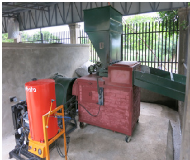
Figure 4b: The Downdraft Rice Husk Furnace Used for Flatbed Dryers in the Philippines.
