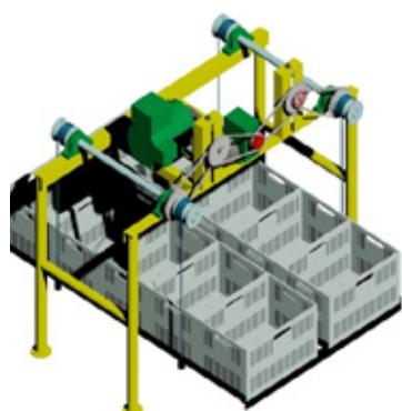
Figure 16: Rendered View from an Autocad Drawing of the Designed Lifting Device (Yaptenco and De Ramos, 2012).
