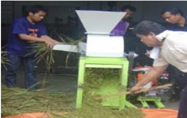
Figure 3: Straw Chopper of 400 kg/h Capacity Has Been Widely Use by Farmer to Provide Cattle and Goat Feed.
