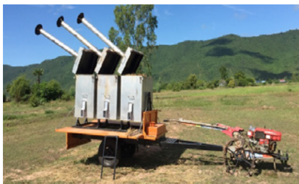
Figure 3: The Picture Shows the Mobile 3 Chambers TULD Kiln Fixed on Trailer and Towed by Power Tiller.
