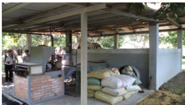
Figure 3: Flatbed Dryer Using Rice Husk Furnace.
