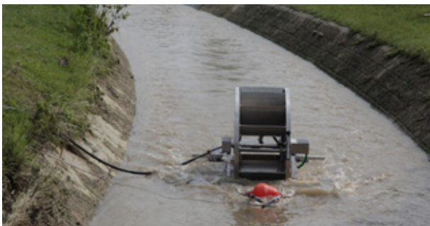
Figure 2: Papa Pump (Hydraulic Ram)
