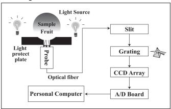
Figure 4.6. Measurement of half transmittance
